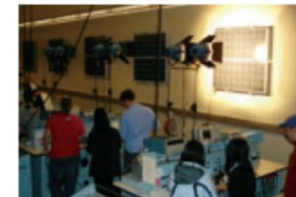
Students in EE 351 use a thyristor controlled dimmer to explore the effect of light intensity on solar cell performance in the Energy Systems Laboratory of the current EE building.
