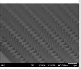
An electron microscope image of an array of silicon nano-pillars, made by e-beam lithography and silicon ICP etching, in the Fluke Hall cleanroom. Silicon nano-structures such as these are used in many research projects at UW, including basic research in materials and physics, optics, and bio-mechanics.
