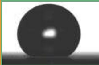
CONTACT ANGLE MEASUREMENT OF A DROPLET WITH VOLUME  $7.68 \mu\text{l}$  LEADS TO  $\theta_r = 137^\circ$  AND THE VOLUME OF DROP IS  $7.68 \mu\text{l}$ . ONE CAN OBSERVE LIGHT BELOW THE DROPLET, CONFIRMING THE HYPOTHESIS THAT THE DROPLET RESTS ON NON-FOULING HYDROPHILIC PILLAR TOPS.
