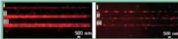
FLUORESCENCE PATTERNS OF 500 NM AND 100 NM WIDE WAVEGUIDES. (A) 500 NM WIDE WAVEGUIDE: I) SINGLE; TWO ADJACENT WAVEGUIDES SPACED II) 200 NM APART AND III) 500 NM APART. (B) 100 NM WIDE WAVEGUIDE - THE RESOLUTION IS DIFFRACTION LIMITED: I) SINGLE; TWO ADJACENT WAVEGUIDES SPACED II) 200 NM APART AND III) 500 NM APART.
