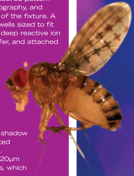
A MICROSCOPE IMAGE OF A FLY, ALIVE AFTER THE COMPLETION OF THE MICROFABRICATION STEPS, WITH AN ARRAY OF 50µM WIDE INDIUM CROSSES ON THE WINGS.
