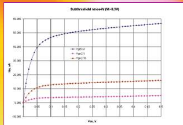
TRANSISTOR SATURATION AT ABOUT 100mV OR (4KT/Q).
