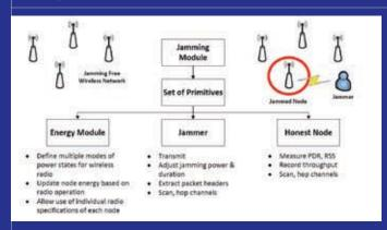
The three primitives defined for the jamming module. The provided primitives are:
