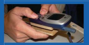
A cell phone body modified for button force sensing. A six-axis force/torque sensor is mounted between masonite plates mounted to the back of the cell phone.
