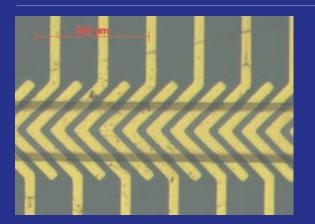
V-shaped electrode arrays were microfabricated and bonded to a cover wafer containing a microfluidic channel. The electric fields generated from the arrays selectively direct particles towards regions of different downstream velocity.
