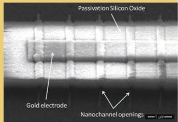
A Scanning Electron Microscope image of the nanochannel sensor.
