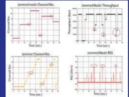
Simulation results showing jamming attack, jamming attack detection and jamming attack mitigation. When jammer is in the same channel as the honest nodes, a fluctuation of network throughput is observed. Once jamming attack is detected, the honest nodes hop to a different channel to avoid the attack. The jammer also reacts to honest nodes' mitigation by scanning all channels for signal and jam on a new channel.
