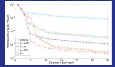
The reweighted heuristic helped identify a low-order dynamical system consistent with measured input-output data. This plot shows the decay in the singular values of the appropriate Hankel matrix. A sharper drop indicates a better description of rank of the Hankel matrix and thus the order of the system.
