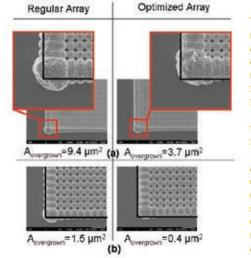
The regular square array (left) and the optimized array (right) are shown for (a) 250 nm seeds with 1.5 µm spacing and 12 seconds growth time, and (b) 500 nm seeds with 10 µm spacing and 60 seconds growth time. The optimized seeds show a sharper corner and a smaller overgrown area.
