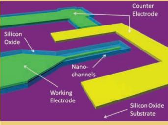
A 3D model of the nanoscale channel biomolecular sensor.
