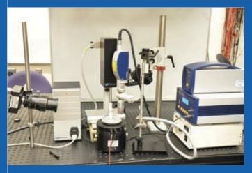
The experimental setup for fluidic self-assembly consists of a high-speed camera, linear electromagnetic vibration exciter, dip coater and laser vibrometer. Thin and fragile parts cannot be handled by pick-and-place robotics, so performing assembly in a fluidic medium is a viable method.
