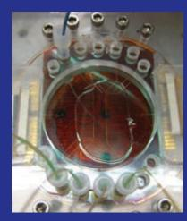
For testing, prototype devices were clamped in a custom acrylic mounting block containing machined vias for microfluidic interconnects. The active device region near the center of the devices is monitored using a fluorescence microscope. However, integrated electric components will use impedance spectroscopy for sensing and detection of particles in future devices.
