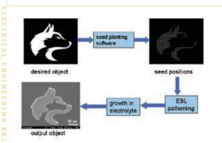
The automated process: the desired object is the input, and the grown object is the output.
