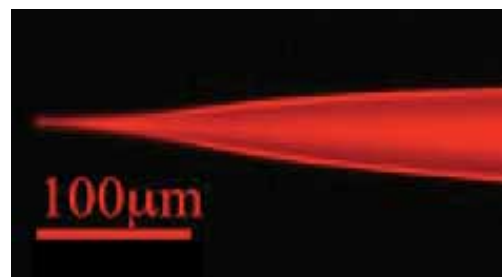
A fluorescence image of a micropipette coated with CdSe QDs.
