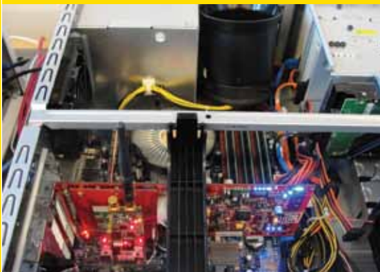
A Sora board embedded into a Quad-Core-CPU PC with XP operating system, which broadcasts the signals on 2.4 GHz and 5 GHz.
