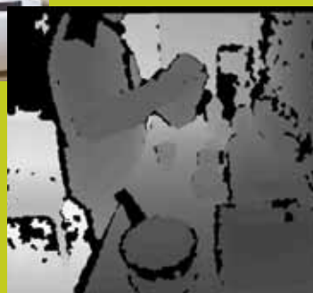
Original color/depth images from the camera. Lighter shades are closer to the camera. Black pixels are sensor failures.
