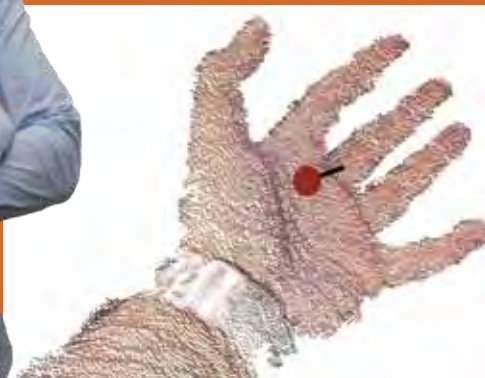
A point cloud of a hand captured by the Kinect camera. The red sphere illustrates the haptic proxy.
