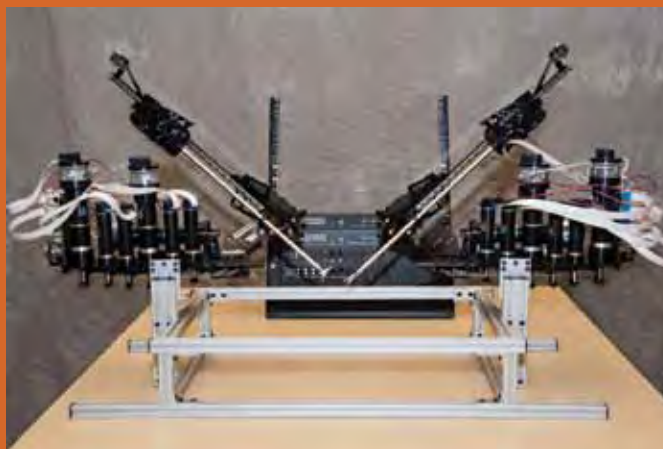
The Raven II's mechanical arms have tiny hands to perform surgery on a simulated patient. In back are the electronics that deliver commands from the surgeon to the robot.
