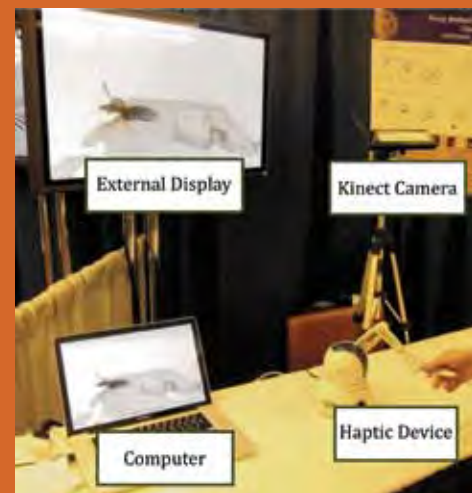
Haptic rendering from time varying point clouds demonstration setup at the IROS Conference in September, 2011. The user moves the haptic device to interact with point clouds captured by the Kinect camera. The haptic rendering runs on a laptop computer and is visualized on an external display.
