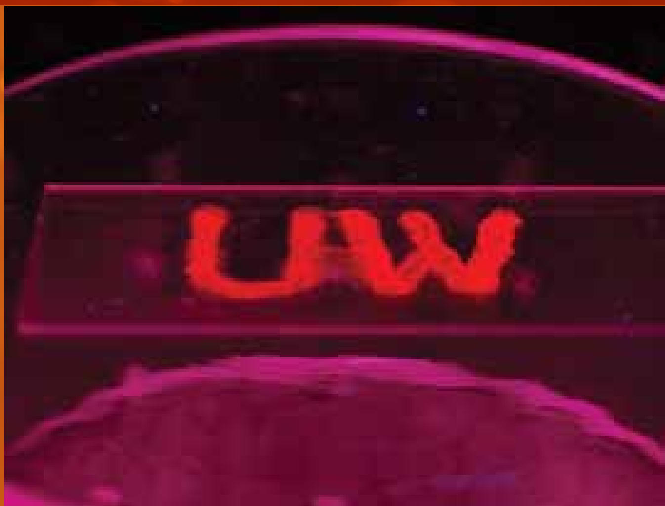
"UW" written by printing with the red-light-emitting SiQD-phosphors on a glass side. The photograph was taken under 365 nm UV illumination.
