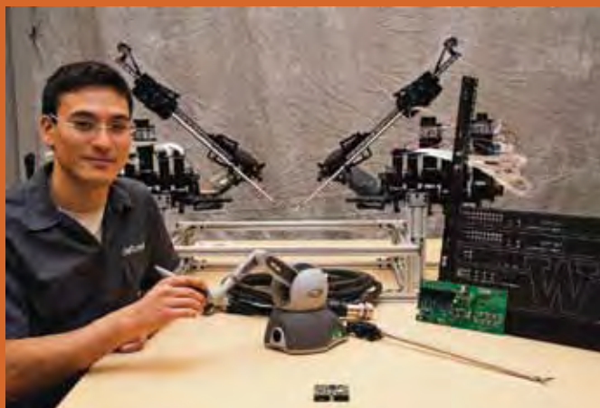
UW EE doctoral student Hawkeye King demonstrates how a surgeon watching a screen would operate the controls. The electronics package (right) would then send those controls to the Raven II robot (center).
