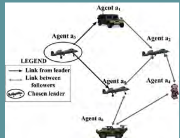
An example of a MAS consisting of networked vehicles controlled by a ground operator.
