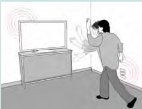
Radiated electromagnetic noise received by the human body enables whole-body gesture interaction with computers.
