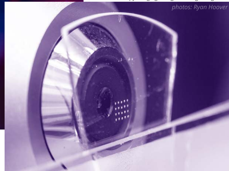
(below) Close-up array of metasurface lenses (metalenses) used for full color imaging, depth sensing, microscopy imaging and generating holograms.
