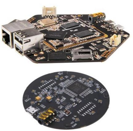
A microphone array is used to collect audio, the array allows for spatial information to be collected. The direction of arrival of the signals assist in noise reduction and speaker identification. Beamforming takes the direction of arrival so that sounds from different directions can be suppressed (noise) or enhanced (speakers).
