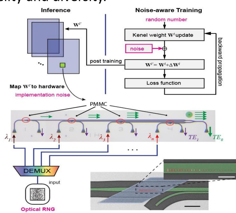
The realistic hardware noises including short-term programming inaccuracy (write noise) long-term measurement fluctuations (read noise)
