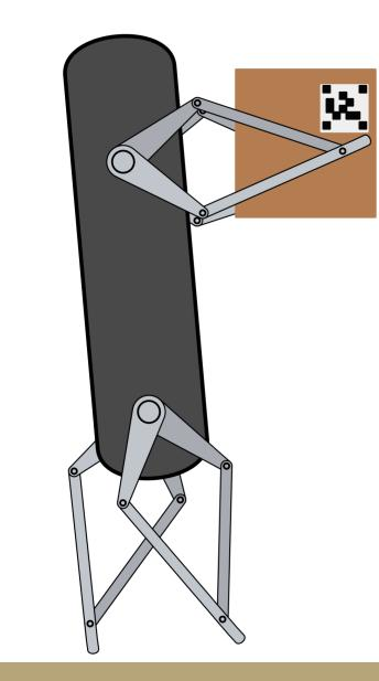
Example concept: a 4-limbed robot which performs tasks in bipedal and quadrupedal configurations. Each limb gets repurposed in the different behavioral regimes.
