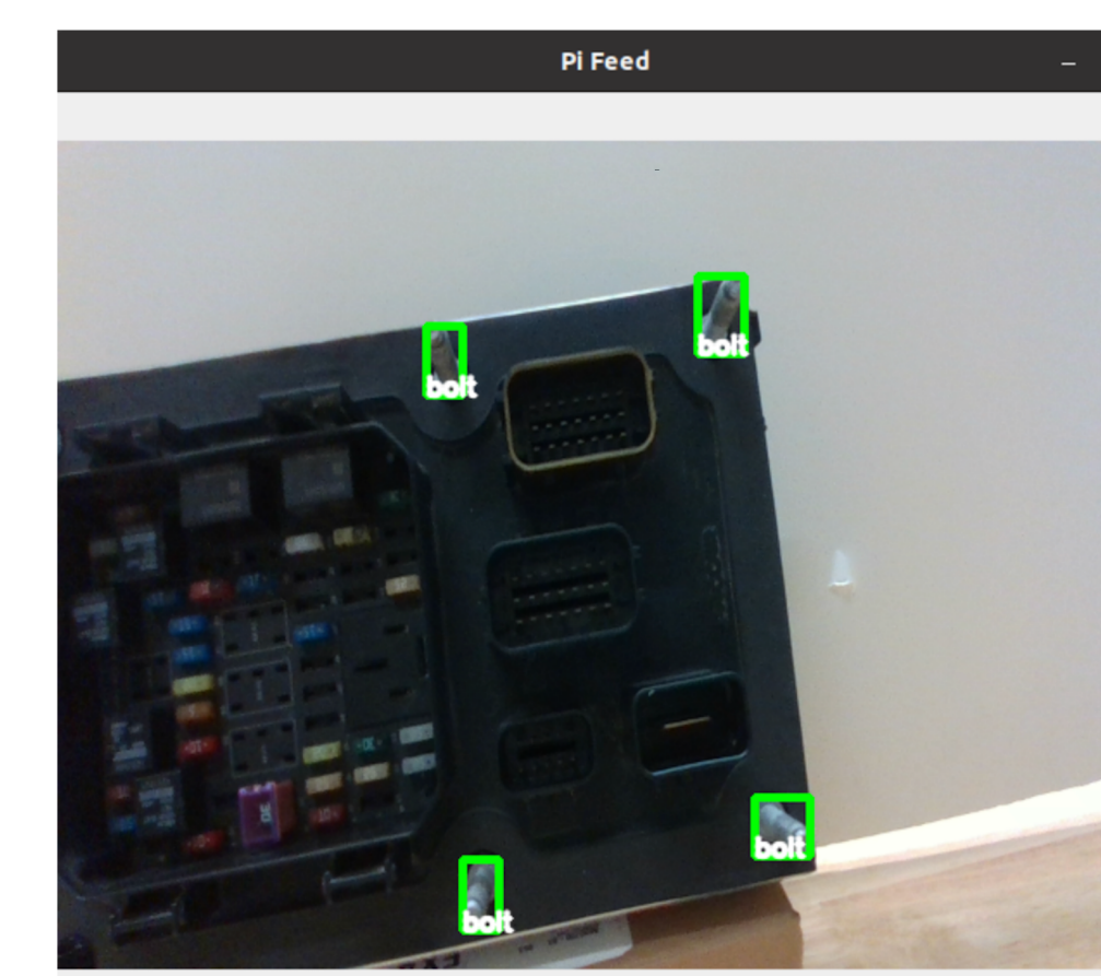
Fig. 7: Bolt Detection Model Test Visualization
