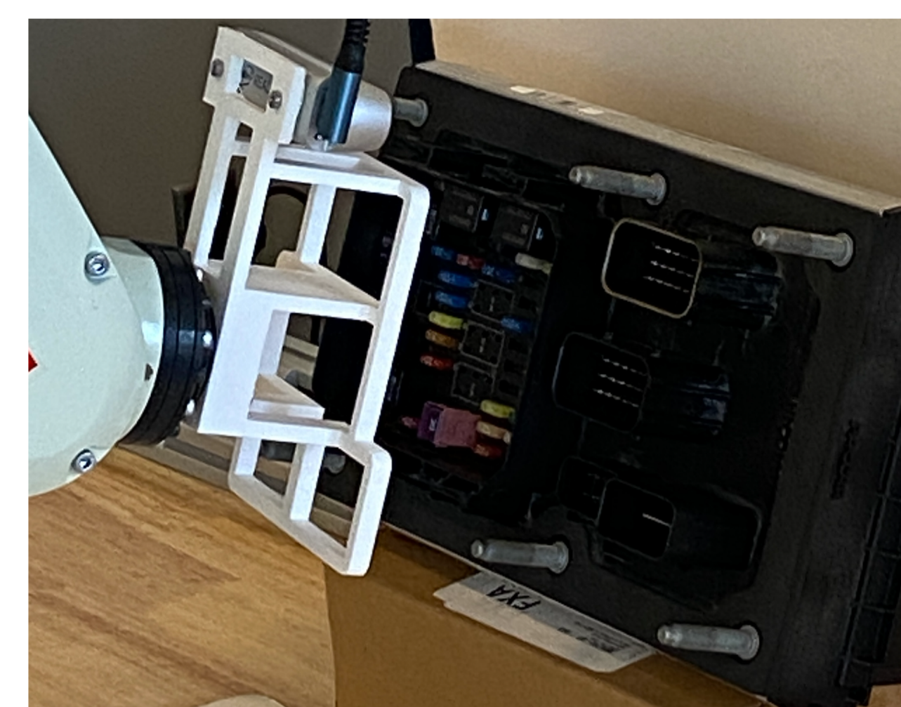
Fig. 6: End Effective Link Position After Dashboard Pose Estimation (Uncalibrated)
