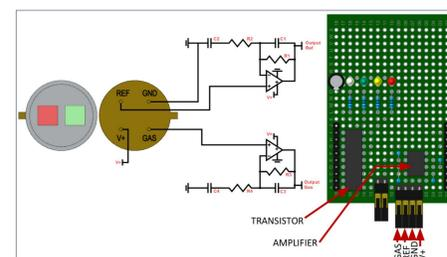
Figure 7: Bandpass/amplifier and DMOS based circuit
