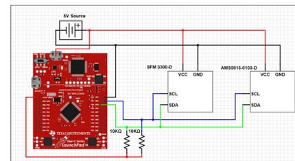
Figure 4: Pressure and Flow Subcircuit
