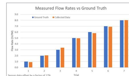
$$flow [slm] = \frac{measured\ value - offset\ flow}{scale\ factor\ flow}$$
