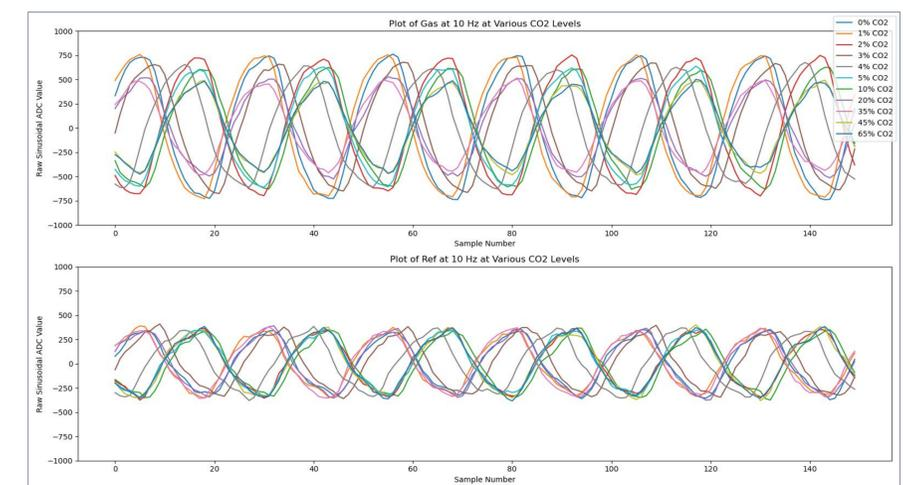
Figure 8: Data plots for gas and reference values from the TM4GX123 ADC (analog-to-digital converter)
