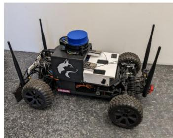
Fig. 4 (above, right): The MuSHR car using four ESP32s
