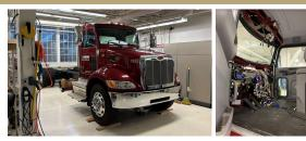
PACCAR provided a Class 7 Peterbilt 337 for us to convert. The diesel engine, as well as the Alison transmission, the driveshaft, and most accessories had already been removed. Four inches of frame rail was cut to fit the truck into our shoo.
