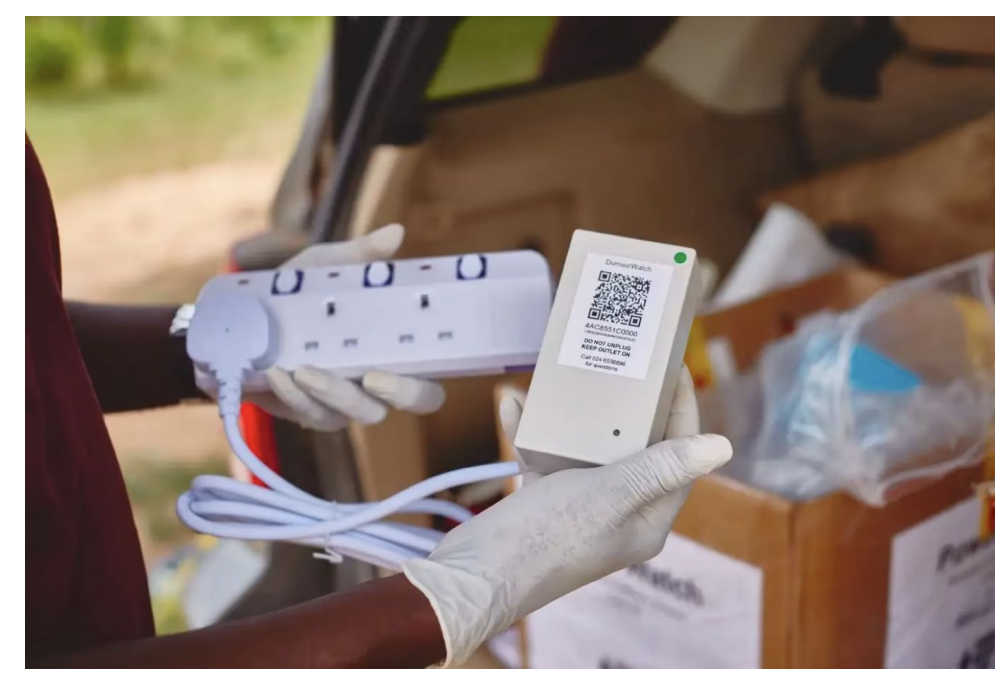
Figure 2: The PowerWatch sensor plugs into a customer's electrical outlet and measures power quality & reliability data every 2 minutes.
