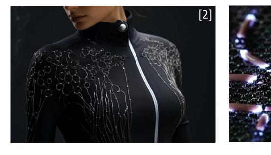
human-machine multifunctional textile-based interface enables The bidirectional interaction while ensuring wearability. In our work, we developed a wearable system that achieves sensing human body movements and providing corresponding haptic feedback based on a unified structure.
