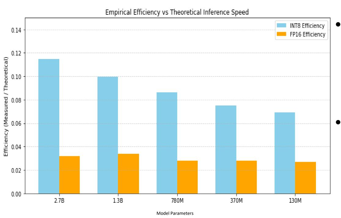
Theoretical upper bound for inference speed vs. our measured data shows that our INT8 quantized model has higher efficiency than the un-quantized FP16 model.
