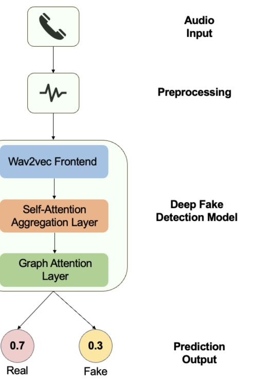
flow Overview: User telephone is preprocessed (segmentation resampling) and then passed to the T2 model to predict the probability of being real or spoofed.
