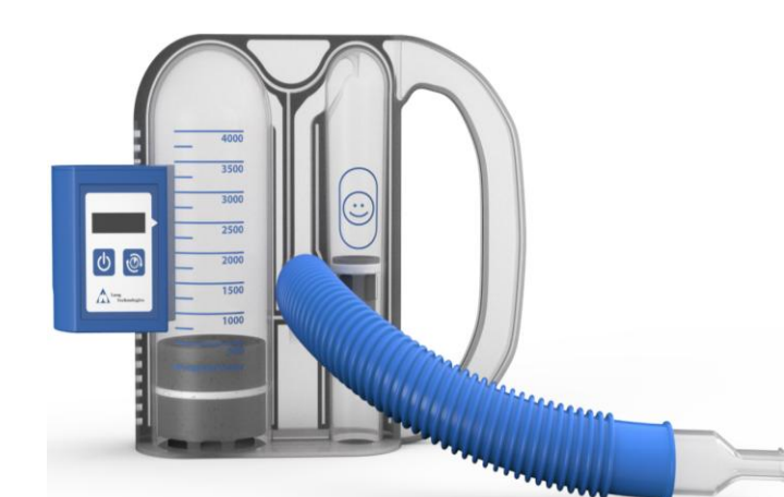
Fig 2. Concept of redesigned incentive spirometer with monitoring device
