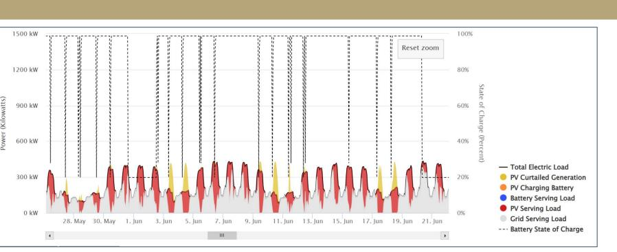
The REopt platform, run by NREL, evaluates the economic viability of distributed energy resources (DERs) for the microgrid, as well as strategies to mitigate the cost and achieve resiliency within the system. This simulation displays the potential load profile for the microgrid over 8760 hours, totaling one year in use.
