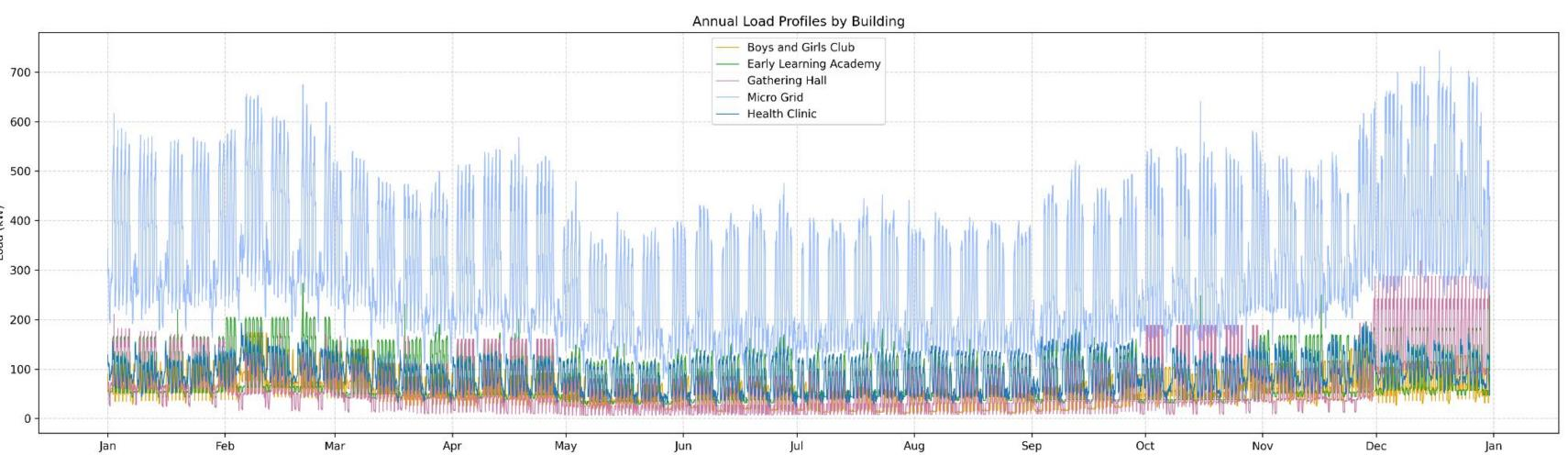
Hourly Load profiles were generated for each building and aggregated into a microgrid profile using the following data from Snohomish PUD Power Trend Analytics Reports (2020-2023):
