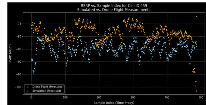
Fig. 13. RSRP Comparison: Simulation VS Real Flight
