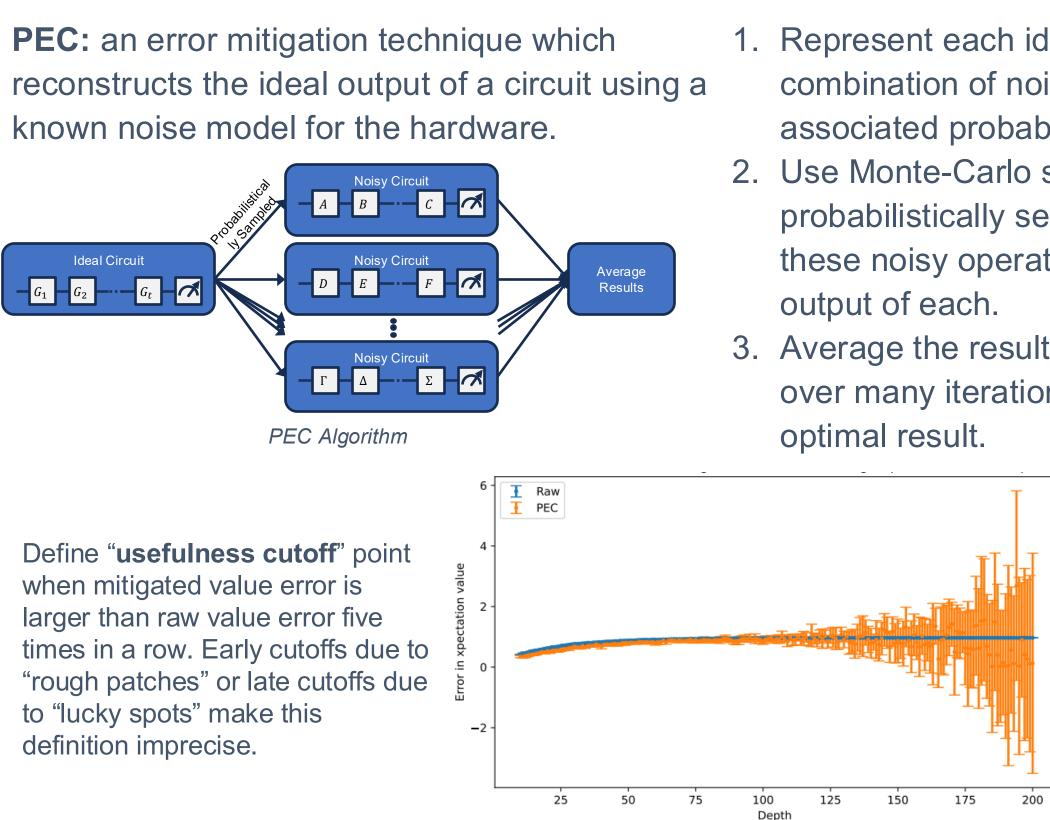
Deeper or wider circuits mean more gates and more possibilities for the sampler to choose from, leading to a greater variance in output values for each run. With a fixed sample number, this leads to larger error bars and a greater change to average to a poor result.
