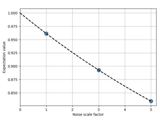
**ZNE:** an error mitigation technique where noise in the form of additional gates are systematically increased without changing the ideal outcome of a measured observable. allowing users to utilize simple statistical methods to find the "zero-noise" limit.
