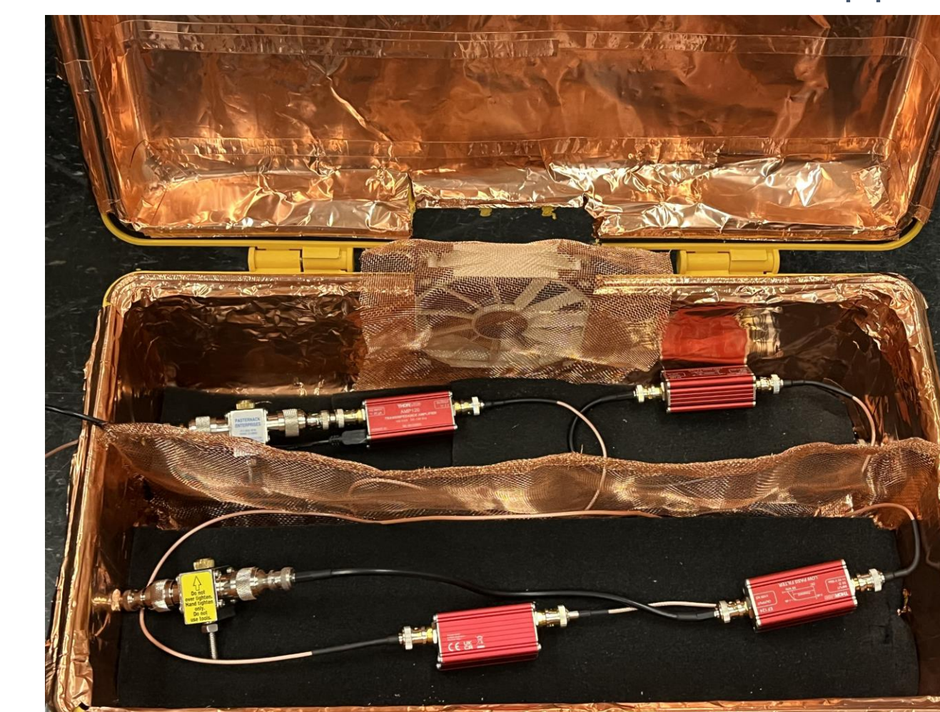
Analog Box with EMI shielding and weather module
