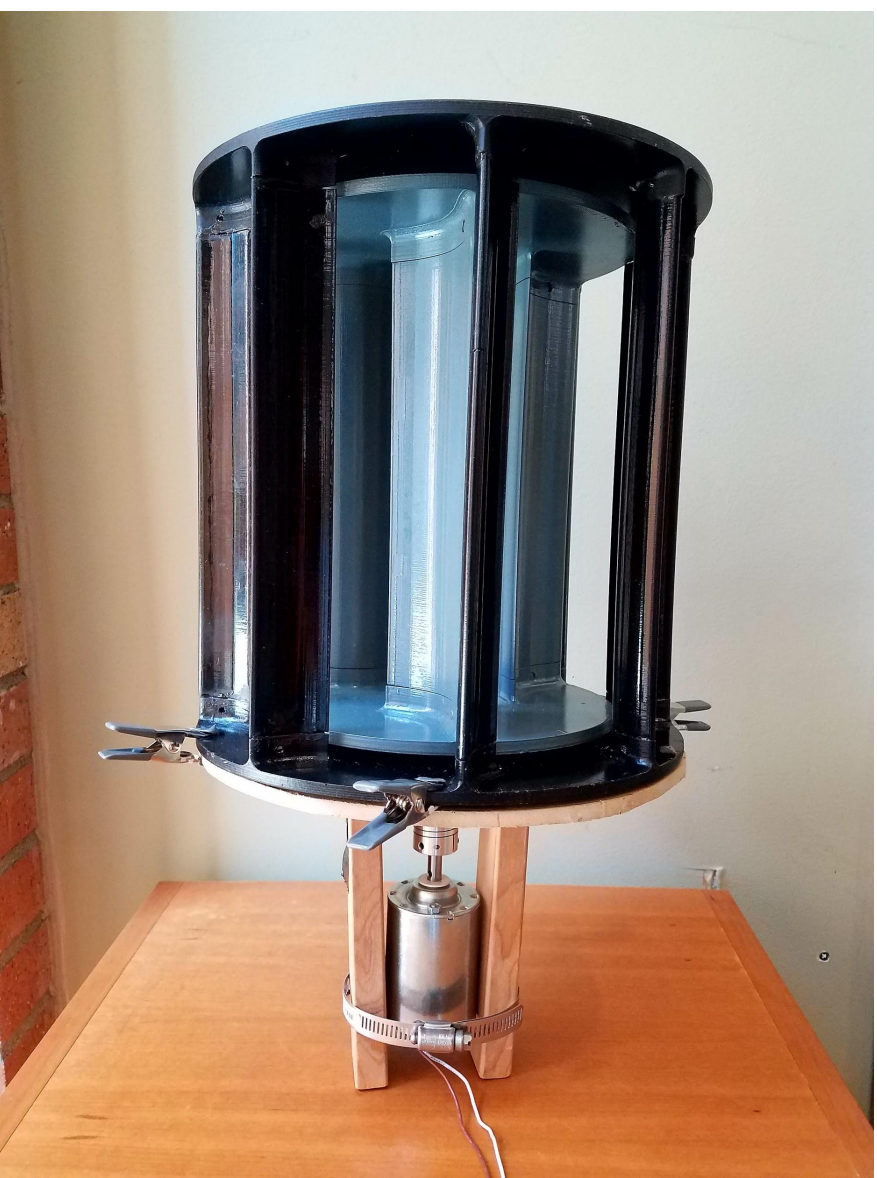
Figure 3B: Wind Turbine Connected to Generator through a coupling
