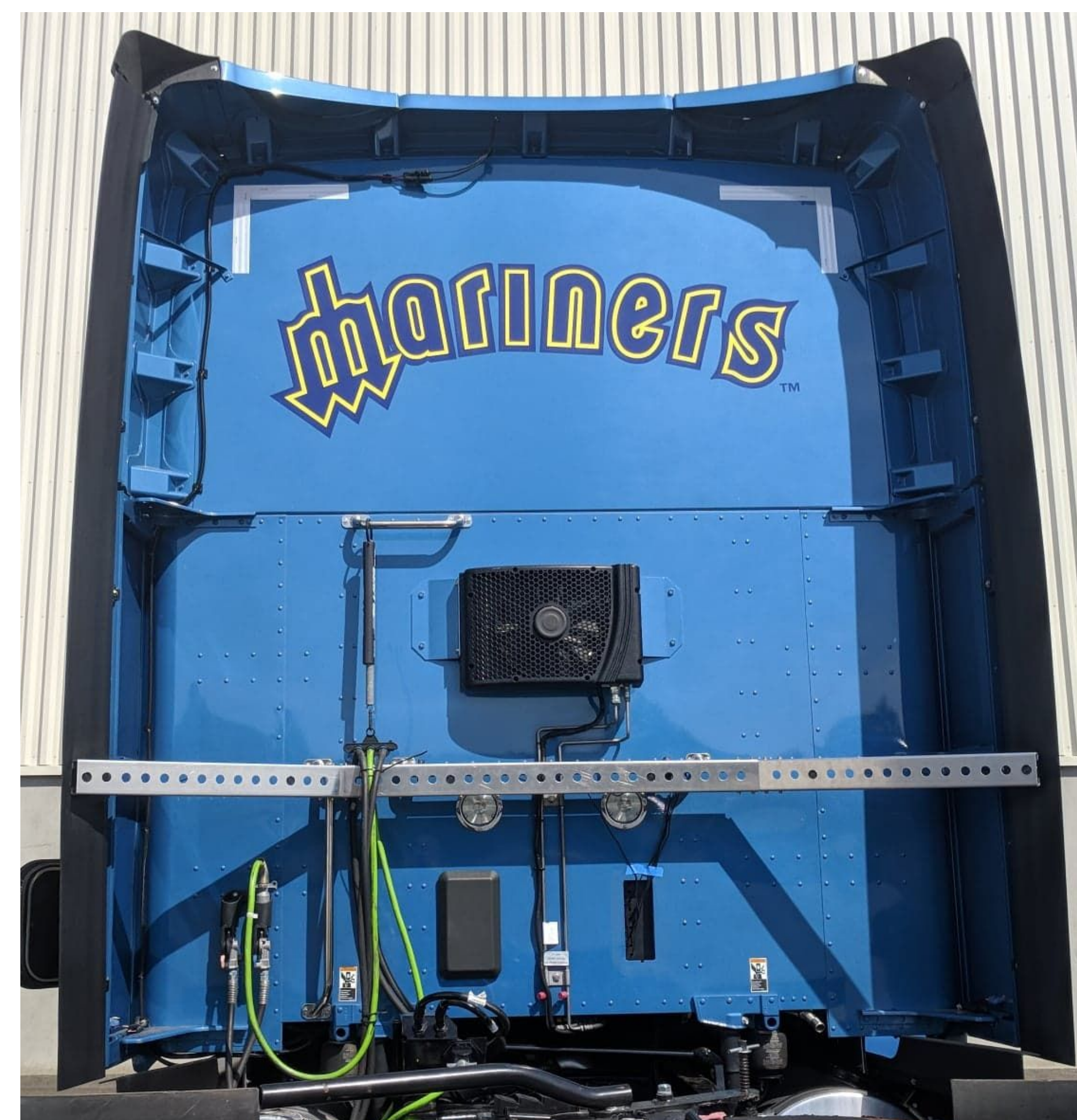
Fig. 2: Ultrasonic mount on Kenworth test vehicle
