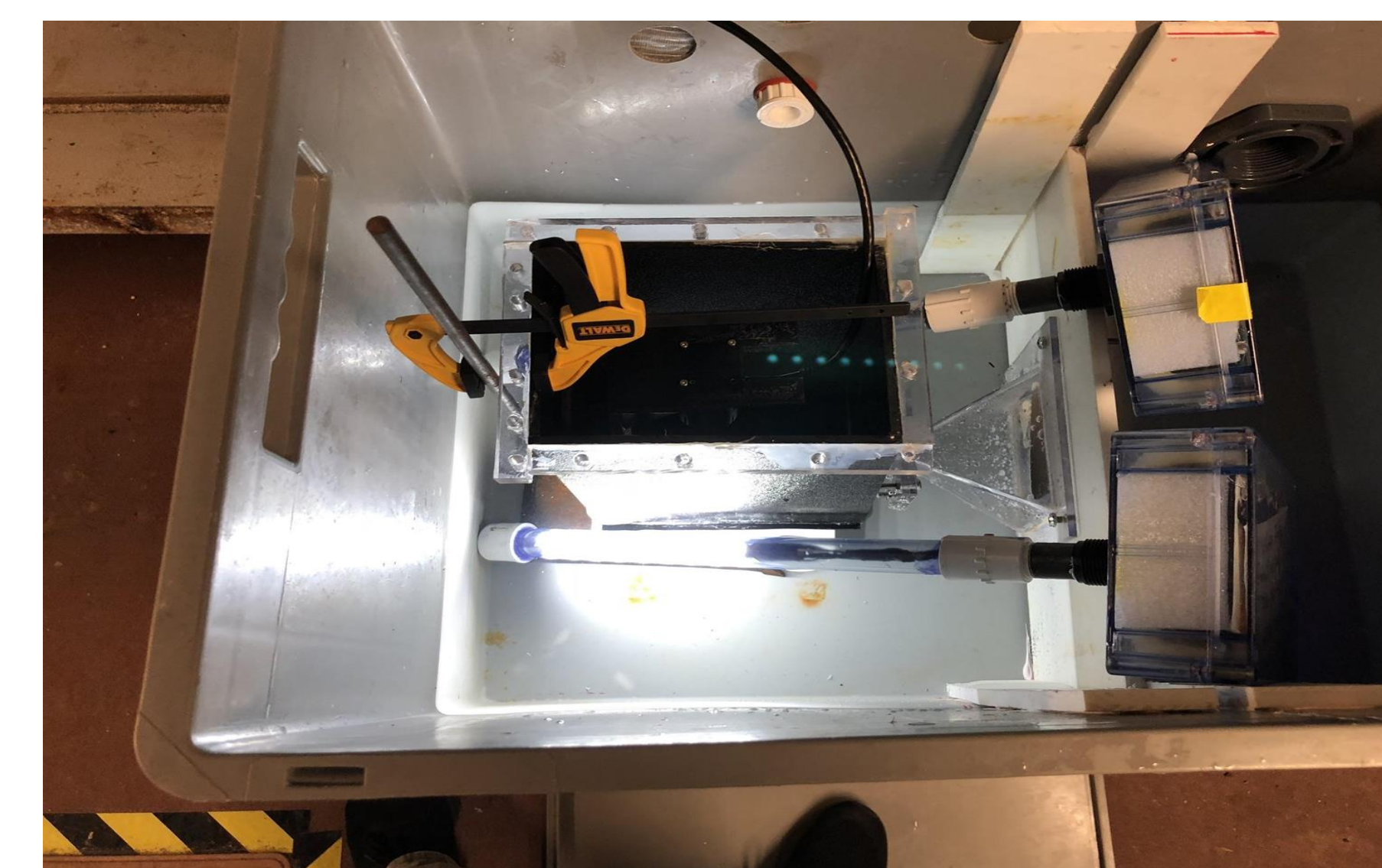
Aquarium setup consisting of the camera system, LED light strips and the sample zooplankton.
