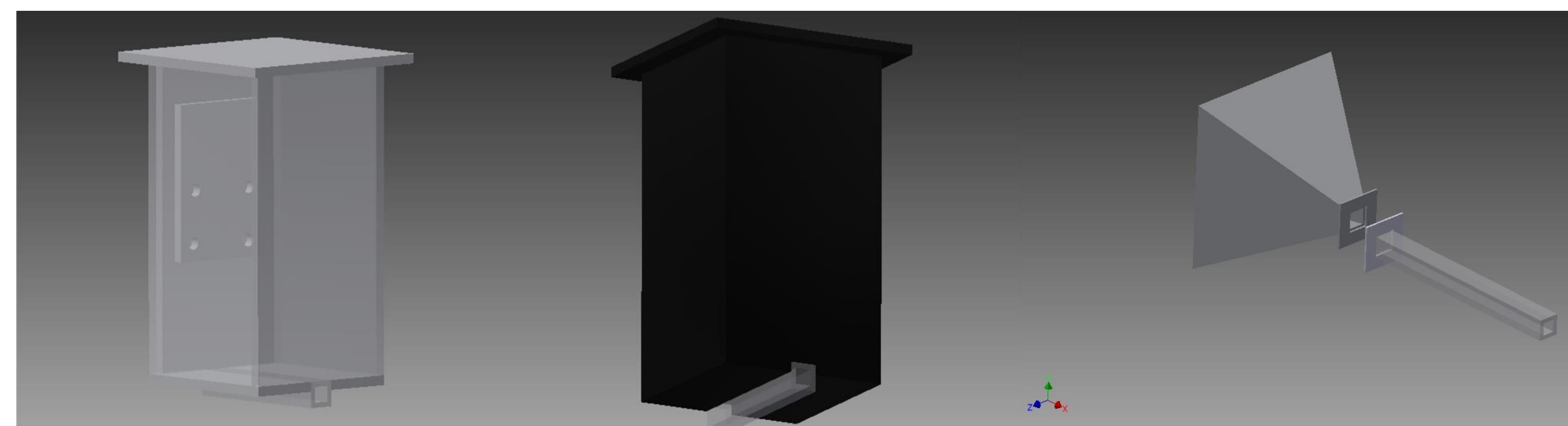
Autodesk Inventor models for camera enclosure, viewing tube, and collection funnel
