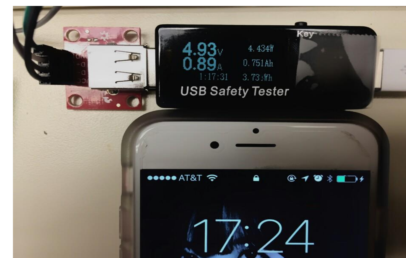
Figure 8. Measurement of voltage (Vbus) and current while charging an iPhone
