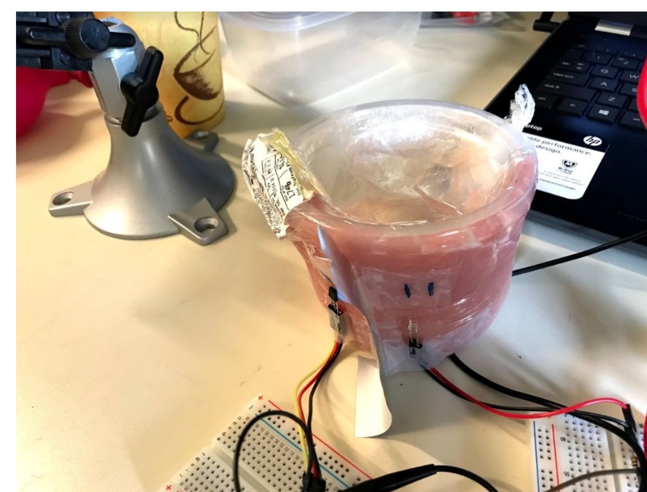
Figure 5: Early test set up with pork, water, and NIR sensors and LEDs
